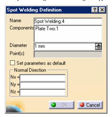
**3.** Select **Plate One** as the second assembly component to be used to create the spot welding.
