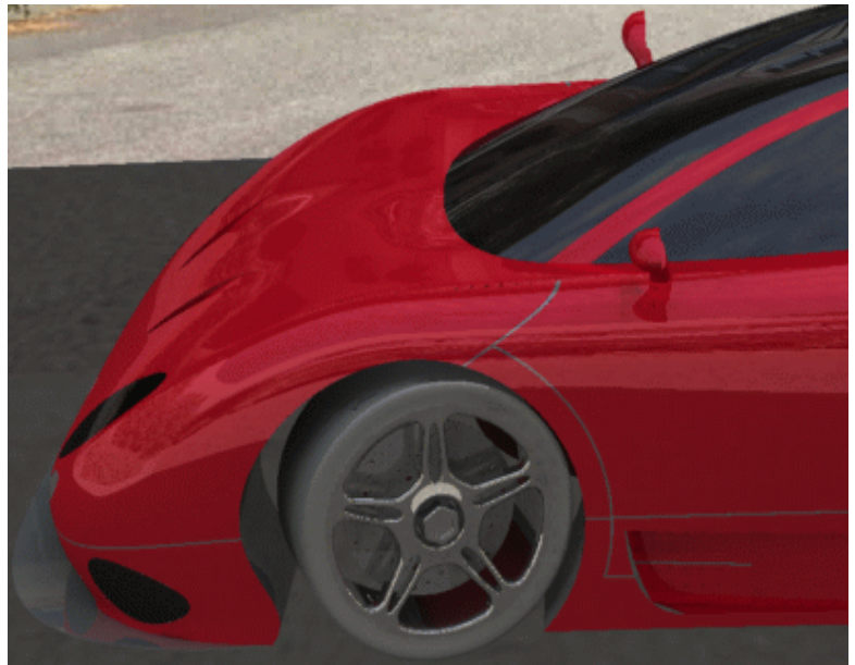
Picture 4 - 5000 rays Maximum radius: 80 Computation time = 5 minutes
