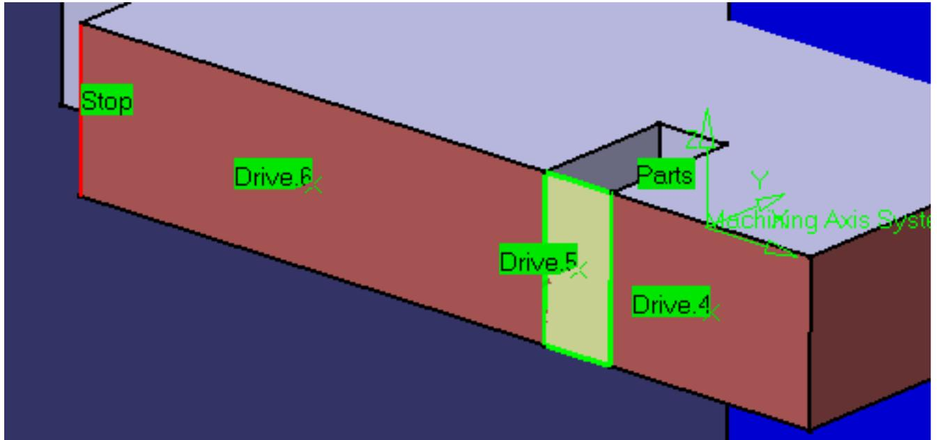
7. Access the Local Drive Surface 4 dialog box and set **Stopping condition** to **Tangent DS**. Access the Local Drive Surface 5 dialog box and set **Stopping condition** to **Tangent DS**.
