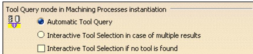
Select the type of Tool Query to be executed when a Machining Process is instantiated:
