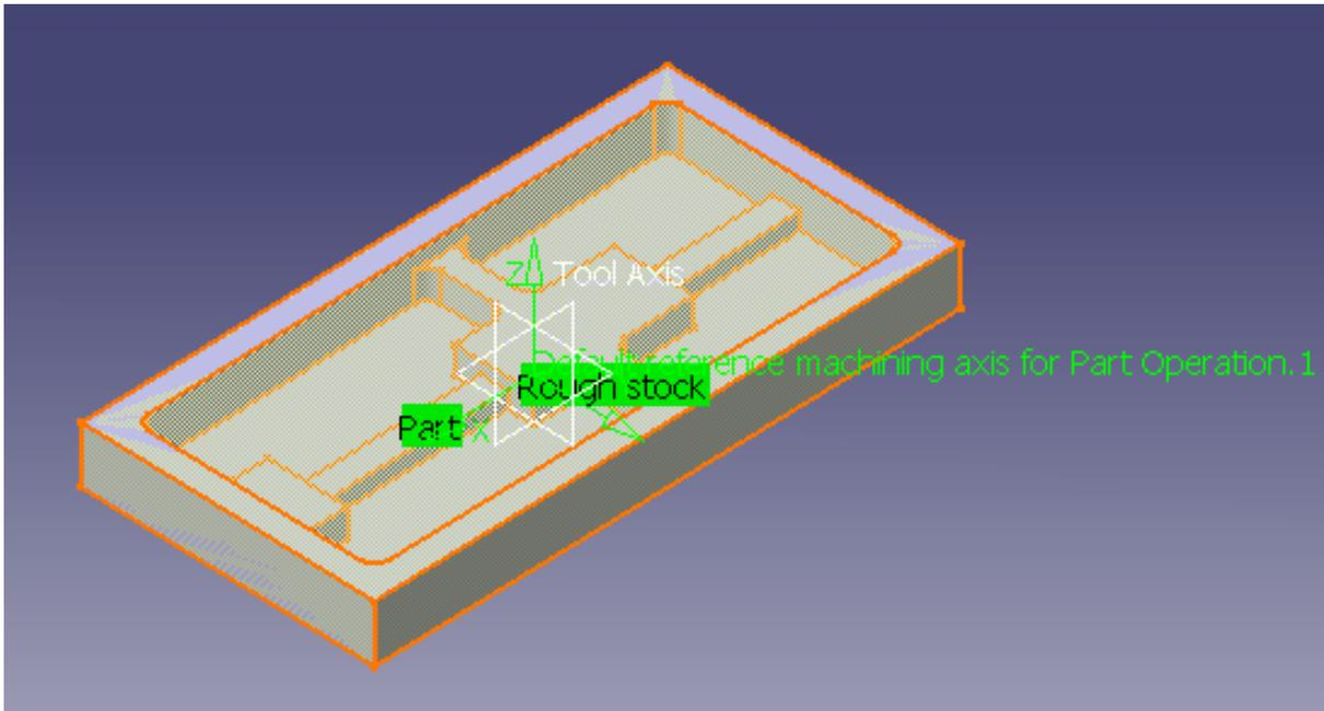
5. Go to the **Machining** tab and make sure the **Machining strategy** is set to Center(1) only.
