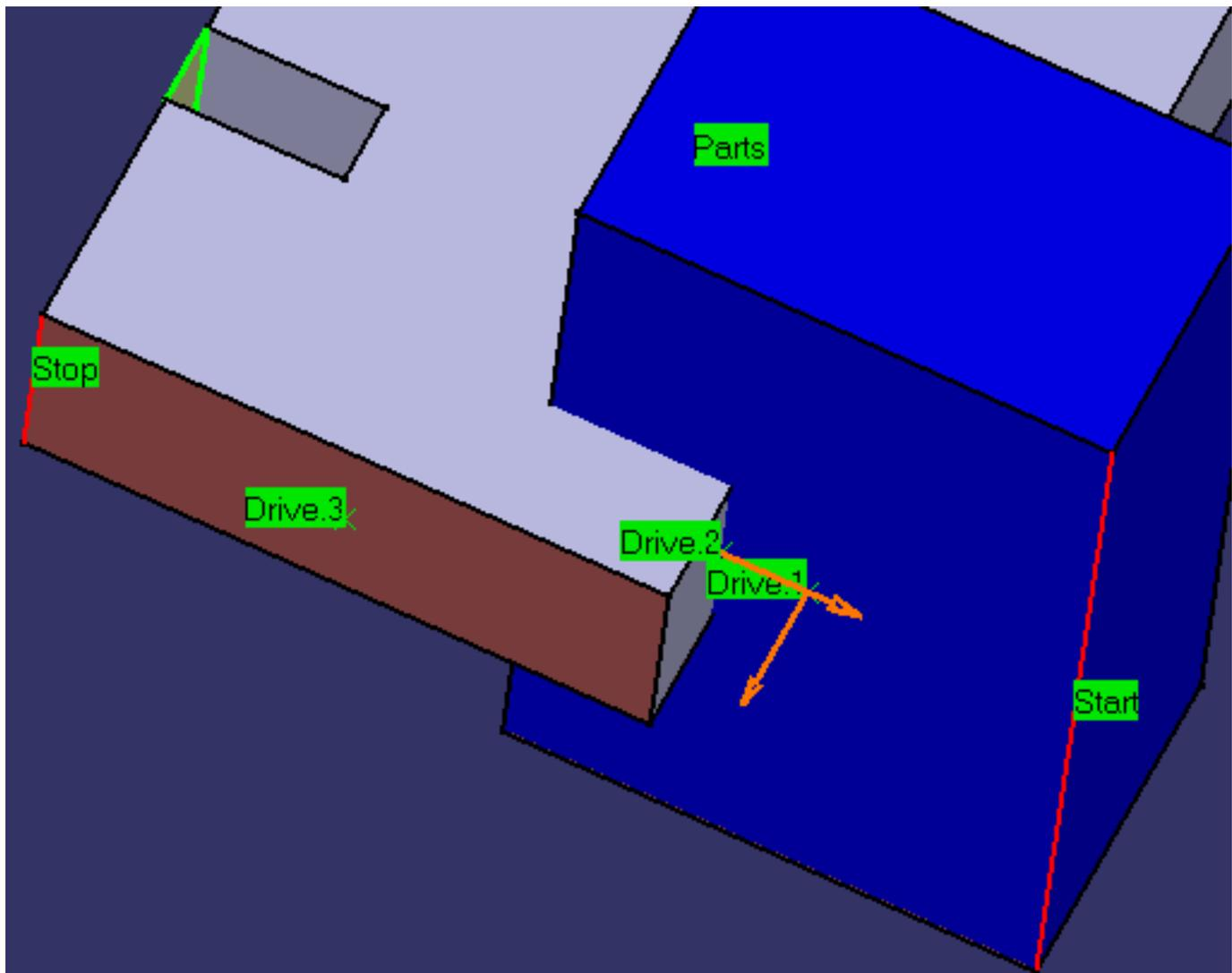
Arrows appear on Drives 1 and 2 indicating the orientation for each contiguous section. Make sure that they are oriented outward.
