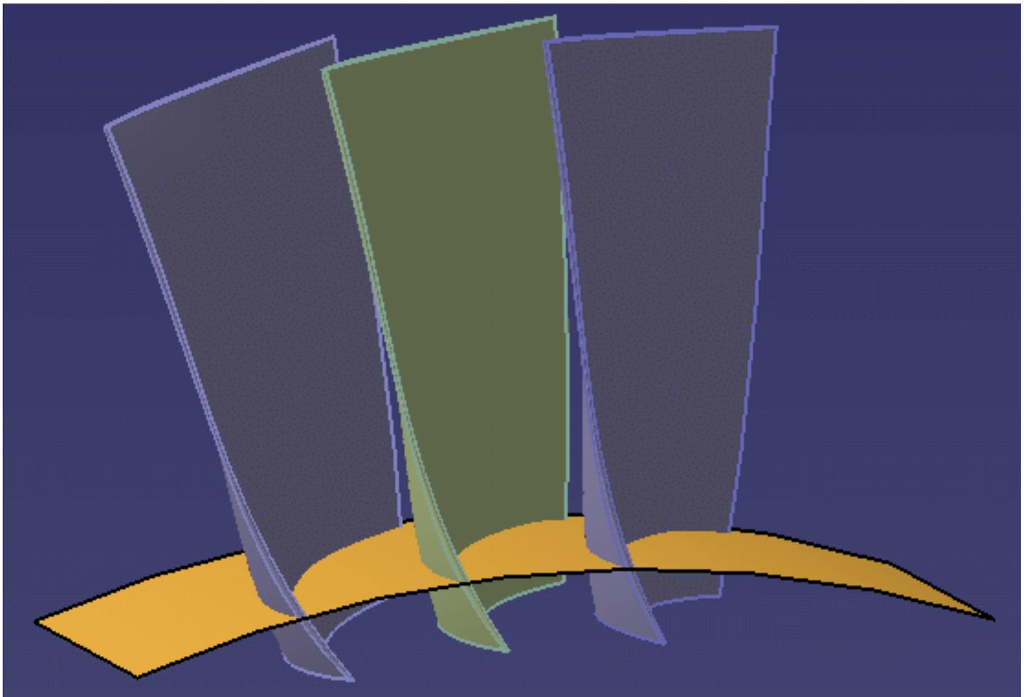
The following procedure describes how to machine the middle (green) blade with no tool collisions with the two neighboring blades.
