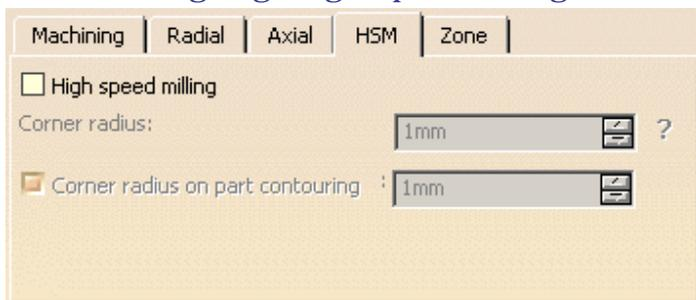
**High speed milling** activates and defines the parameters for High speed milling.
