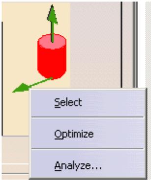
The item **Select** opens a dialog box to select the machining direction:
