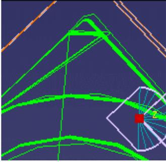
Here is the same tool path with the High speed milling switched on. Note how the round tool path ends. In both cases a concentric tool path style is used.
