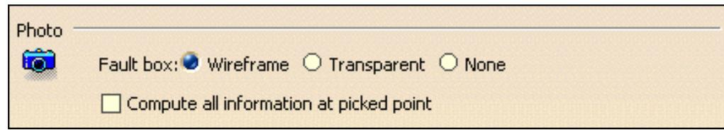
Select the desired **Fault box** type for examining remaining material or gouges:
