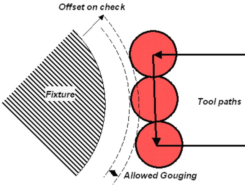
The illustration below shows return motion with macro between path and fixture.
