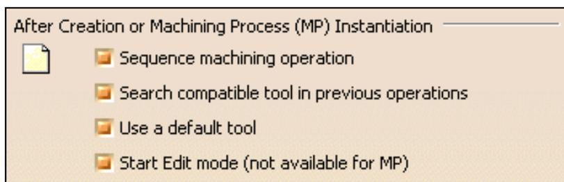
Select the desired checkboxes to specify conditions to be applied when you create machining operations or machining processes.
