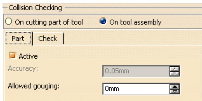
Replay the tool path to check for collisions. At this stage, since there are no selected check elements, collision checking is on the part elements only.
