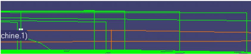
And here is the same tool path with high speed milling switched on:
