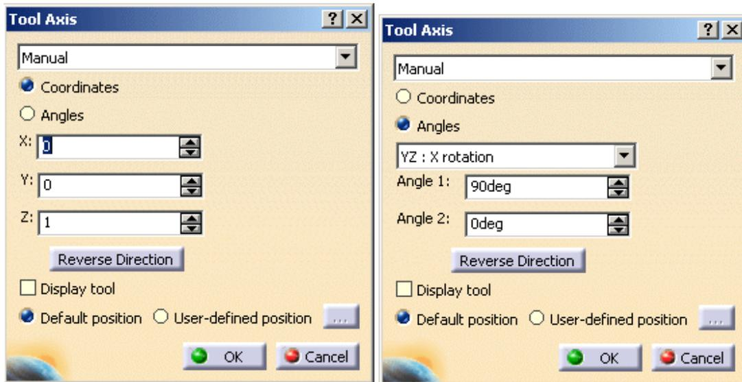
You can choose between selection by **Coordinates** (X, Y, Z) or by **Angles**. Angles lets you choose the tool axis by rotation around a main axis. **Angle 1** and **Angle 2** are used to define the location of the tool axis around the main axis that you select.
