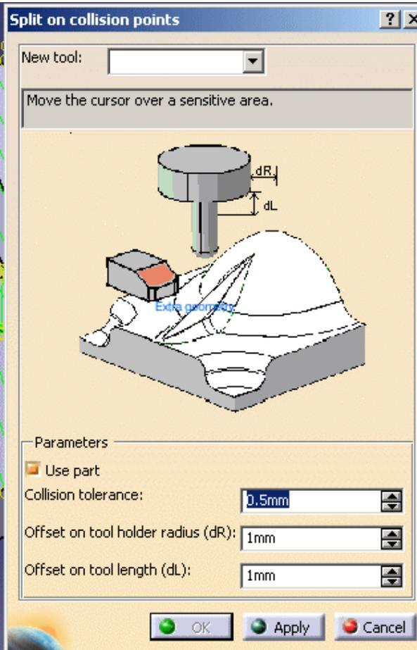
Extra geometry allows you to add additional geometry to the part in the operation where the tool path was computed. Additional geometry may be a face or a clamp that you would rather avoid using in the computation and that is not defined in the operation.
