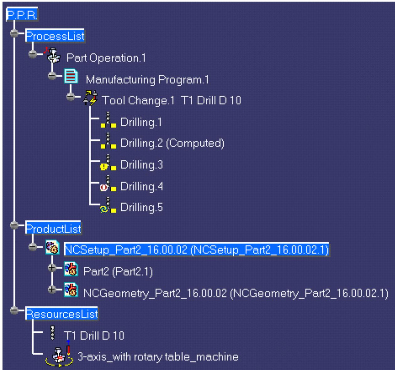
**Process List** is a plan that gives all the activities and machining operations required to transform a part from a rough to a finished state.
