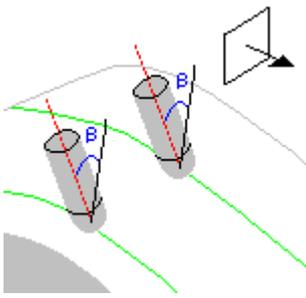
For example, this mode is dedicated to milling parts with tool axis nearly parallel to the part itself (near flank milling). It is primary intended for NC machines whose configuration is A+C, but it can be used on any other multi-axis machine.
