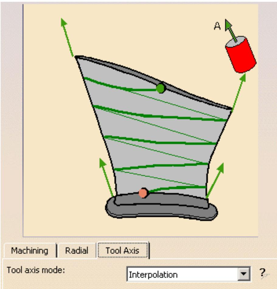
7. Default Interpolation axes (I.1 to I.4) are displayed at the four corners of the part.
