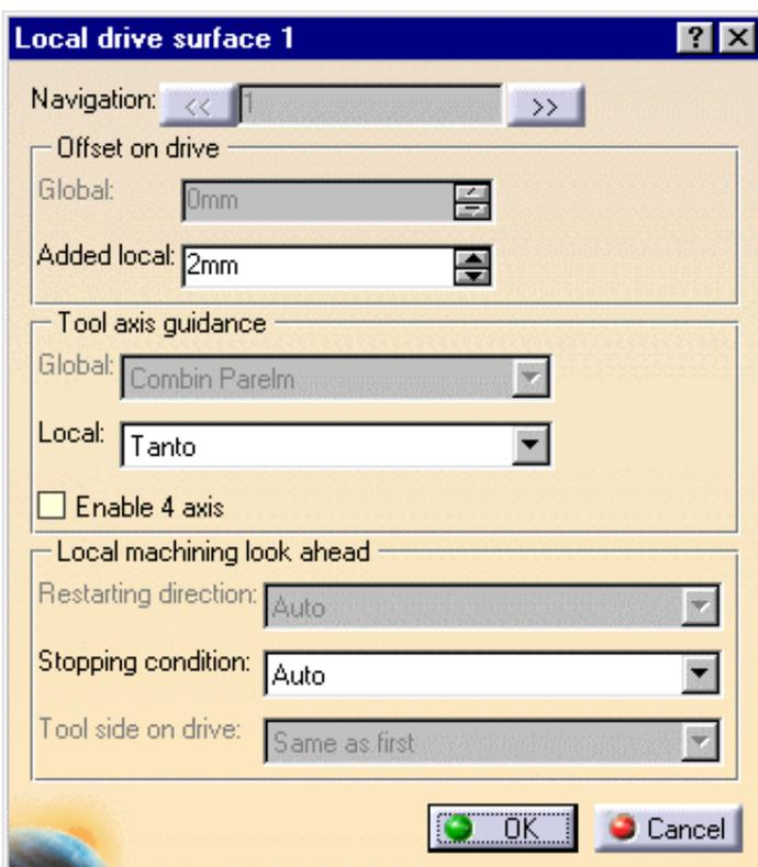
Modify the drive by adding a 2mm offset and changing the tool axis guidance to **Tanto**.
