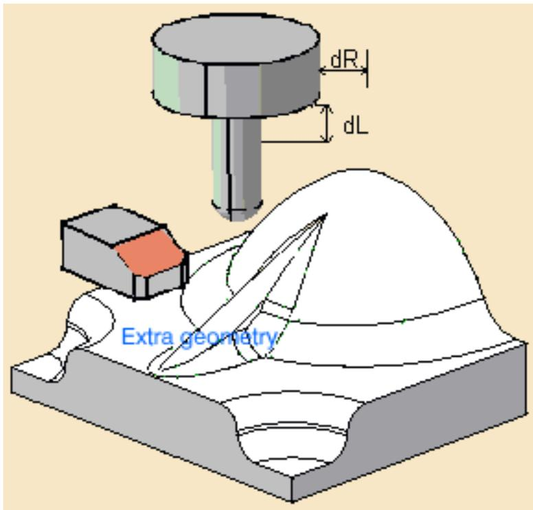
Extra geometry allows you to add additional geometry to the part in the operation where the tool path was computed. Additional geometry may be a face or a clamp that you would rather avoid using in the computation and that is not defined in the operation.
