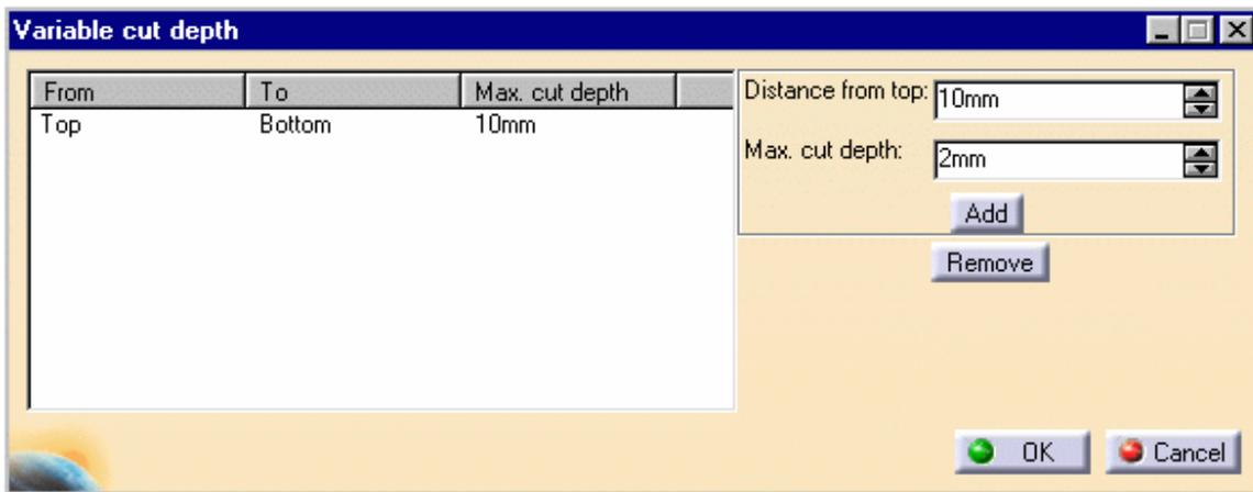
Change the **Distance from top** value and the Inter-pass value and then press **Add** to give a different depth value over a given distance.
