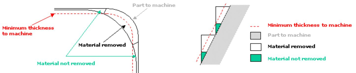
**i** In a given level, the thickness of material left can amount up to the value of the Minimum thickness to machine + twice the value of the tolerance. Therefore, on a level below you may have to mill a thickness amounting to the value of the Minimum thickness to machine + twice the value of the tolerance of one or several levels above.
