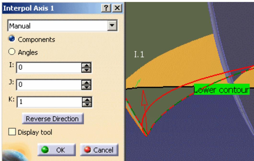
You can select the Display tool checkbox to help you do a rough visual check that the tool is correctly orientated. Note that the tool will be displayed according to the tool tip point (and not the contact point).
