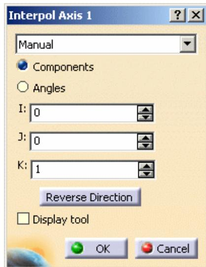
Replay the tool path to verify that the tool can be positioned at each point on the trajectory. If the tool cannot be positioned at each point on the trajectory, you may need to adjust the default axes and/or insert additional interpolation axes. You can insert any number additional axes on the faces of the blade.
