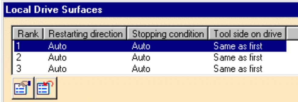
4. Double click line 1, which corresponds to the first drive. The Local Drive Surface 1 dialog box appears. Set the **Stopping condition** to **To**.
