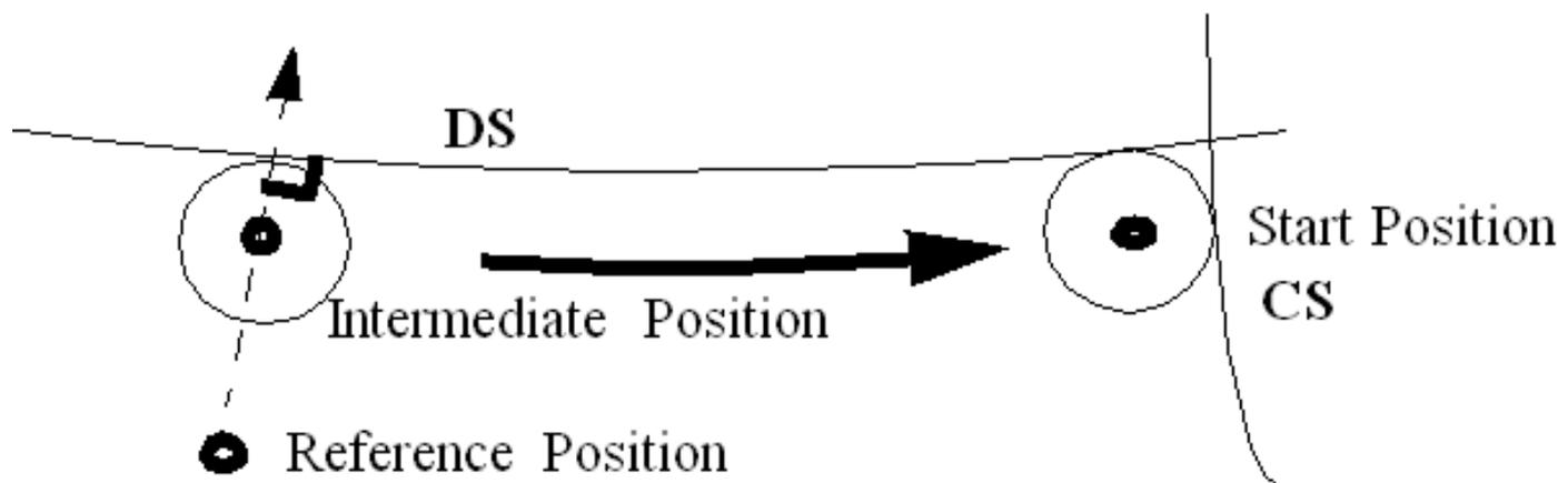
The intermediate position is defined as being the normal projection of the Reference point on the Drive surface.
