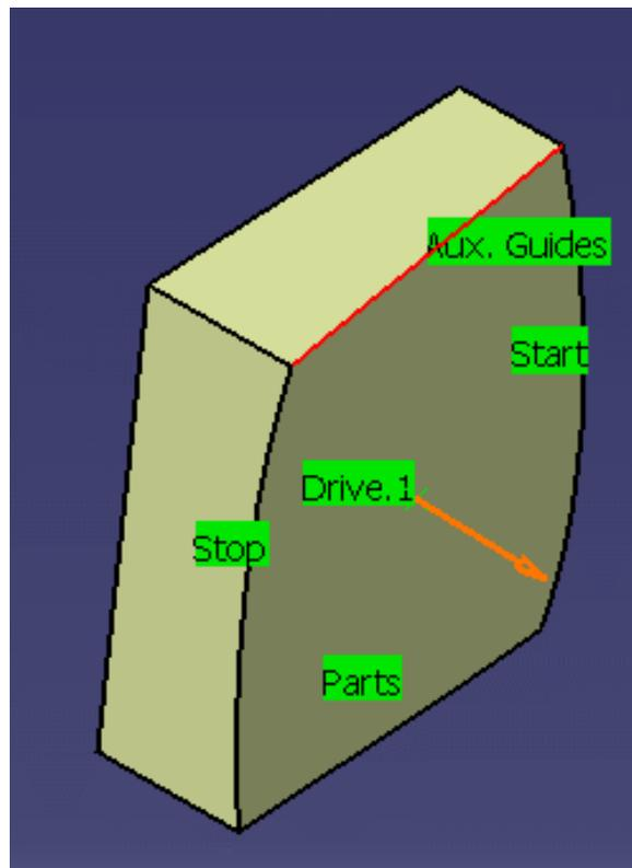
A collision occurs if top auxiliary guide curve is not defined:
