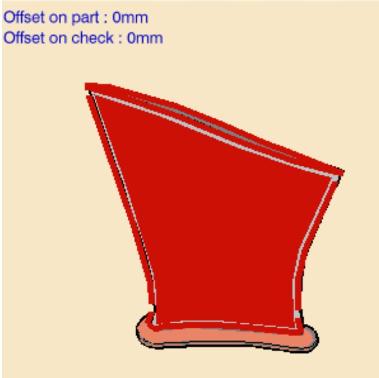
The part surface, upper and lower contours, and leading and trailing edges of the sensitive icon are colored red indicating that this geometry is required and must be selected. The upper and lower contours and the leading and trailing edges must lie on the faces selected as part surface.
