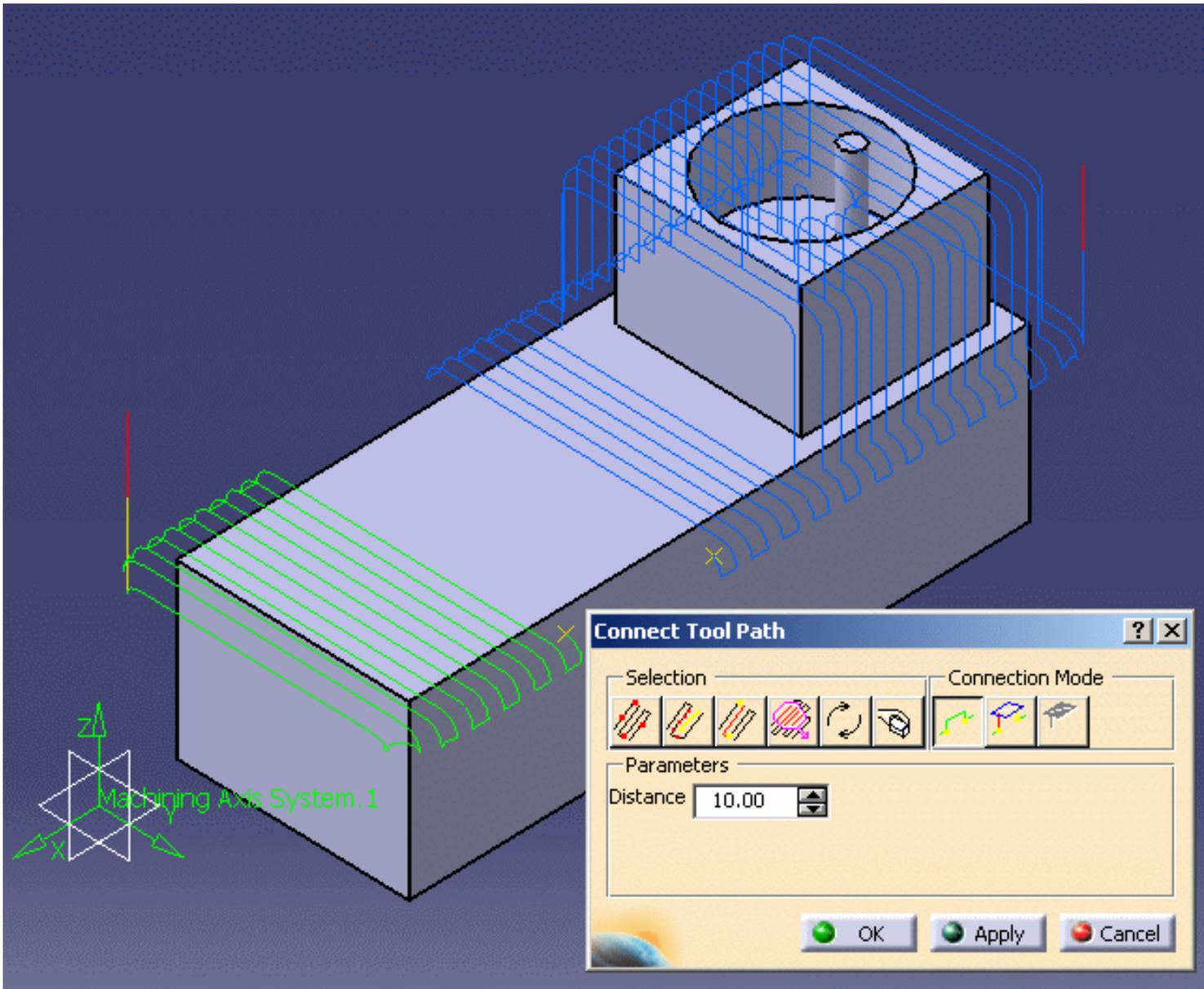
2. Select the points to connect using the **Selection** bar
