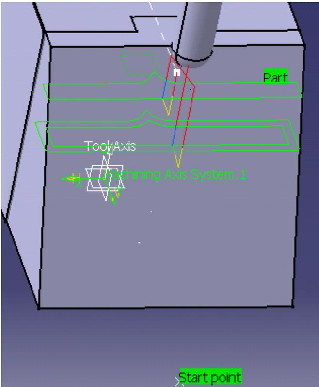
If this is not possible, the path will be cut to respect the constraint imposed by the start point.
