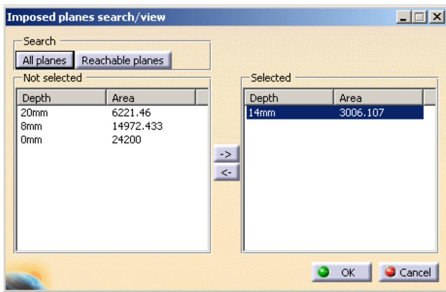
**i** When you are using planar surfaces in a part as imposed surfaces and you are using an offset on the part, select **Offset** in the contextual menu and then enter an offset value that is the same as the offset on part value plus the machining tolerance value, e.g. if the offset on part is 1 mm and the machining tolerance is 0.1 mm, give a value 1.1mm.
