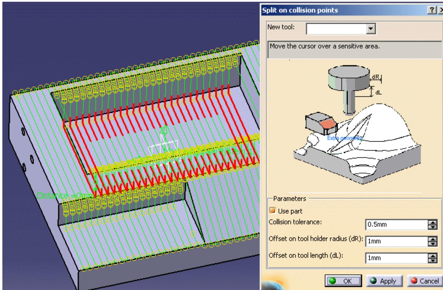
3. Now select a longer tool (T5 End Mill D 10L50) in the **New tool** list:
