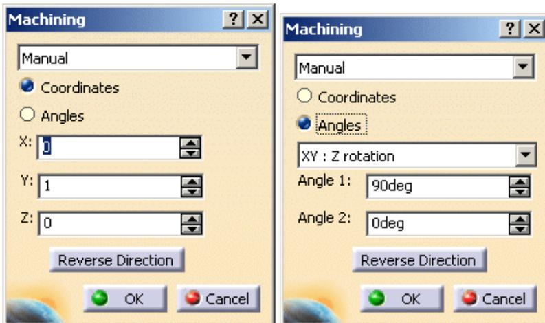
You can choose between selection by **Coordinates** (X, Y, Z) or by **Angles**. Angles lets you choose the machining direction by rotation around a main axis. **Angle 1** and **Angle 2** are used to define the location of the machining direction around the main axis that you select.
