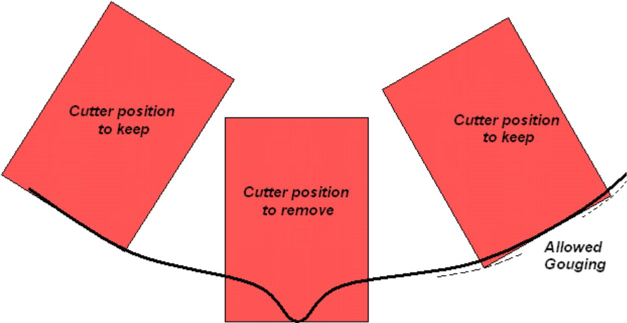
In Multi-axis Helix Machining, collision checking on part elements is **not useful** in the following cases.
