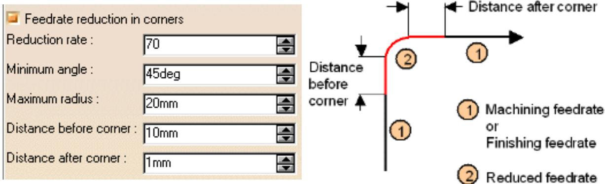
Feed reduction is applied to corners along the tool path whose radius is less than the Maximum radius value and whose arc angle is greater than the Minimum angle value. Corners can be angled or rounded.
