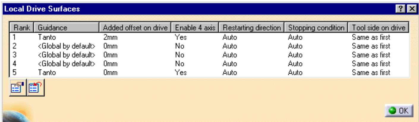
11. Check the validity of the modifications by **replaying the tool path**. The 4-axis constraint is applied on first and last drives.
