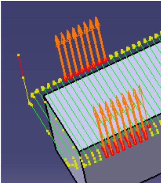
5. Click **Apply**, the axes are created under the Geometrical set **Sweeping.1** . Click **Close** to exit the action
