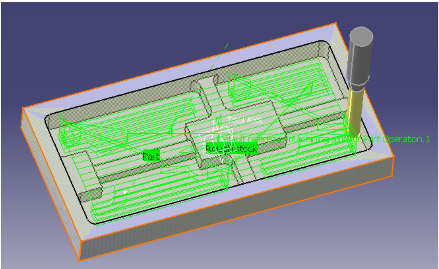
You can see that the tool path direction has been adapted to the geometry to machine, i.e. defined by the shape of each pocket and set along the main direction (X or Y).
