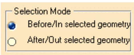
Depending on the button you pick, you can choose whether the part of the tool path selected is before or after the single point or inside or outside the two points or contour. Whichever of the buttons you choose its effect will be applied to the next tool path selection action.
